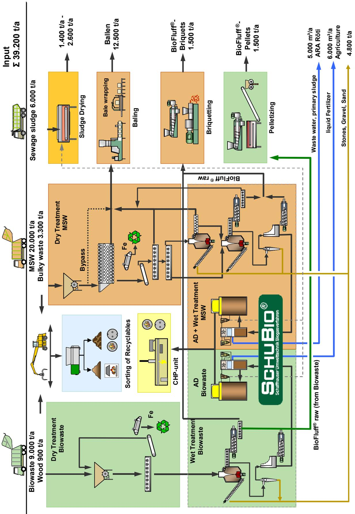
Figure 3: Process Flow Diagram KBA Hard with SCHUBIO®-Process
